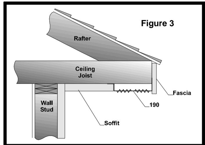
***It must be noted that the 190 soffit vent will only ventilate your attic if it has a clear air passage, therefore it will be necessary to ensure that attic insulation as well as any other materials do not block your vents air passage.***
