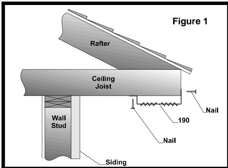
In most cases, it will be necessary to cut a section of vent to install the final section. The cut should be made with tin snips. Measure and cut your final piece so that the factory edge will butt against the fascia board and the end you have cut will go under the adjoining section by at least  $\frac{1}{4}$ ".
