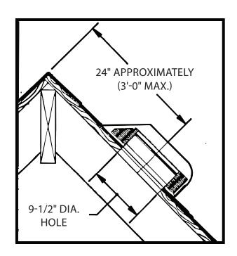
5. Starting in the drill holes cut two 9 1/2' diameter circular openings, using either a keyhole saw or an electric saber saw with sharp coarse blade. If you do not have a coarse blade, cut away shingles inside the circle with utility knife before cutting roof decking. Take care not to make the holes too large or water leakage may occur.
