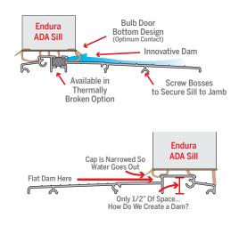
Endura's patented dam feature provides the most effective method for preventing air and water infiltration.
