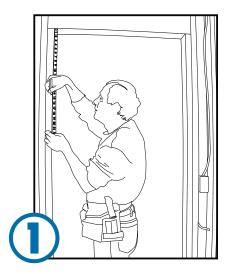
Frame in opening in the usual way, then measure down half the width of the arch.
