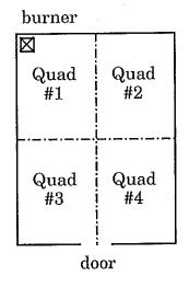
Room Quadrant Thermocouple Locations (Plan View)
