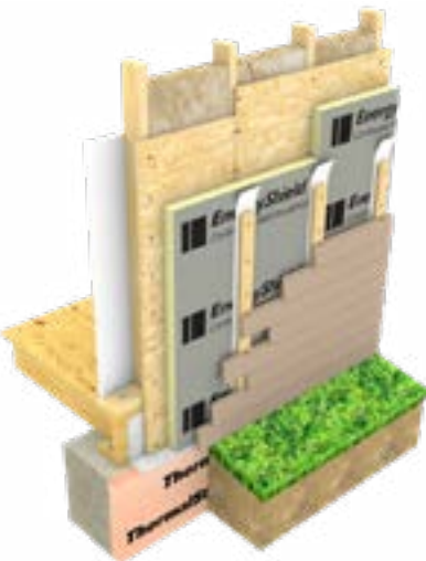
Wood studs, batt cavity insulation, wood sheathing, taped joints, EnergyShield, wood battens, fiber-cement siding.
