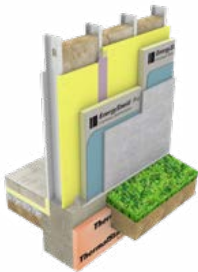
Steel studs, batt cavity insulation, glass-mat faced sheathing, EnergyShield Pro, liquid-applied air and moisture barrier, fiber-cement panel cladding.
