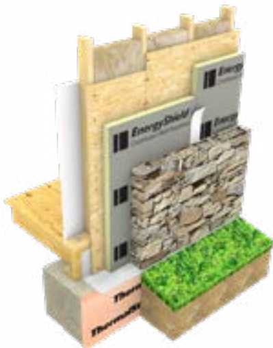
Wood studs, batt cavity insulation, wood sheathing, EnergyShield with taped joints, stone cladding.
