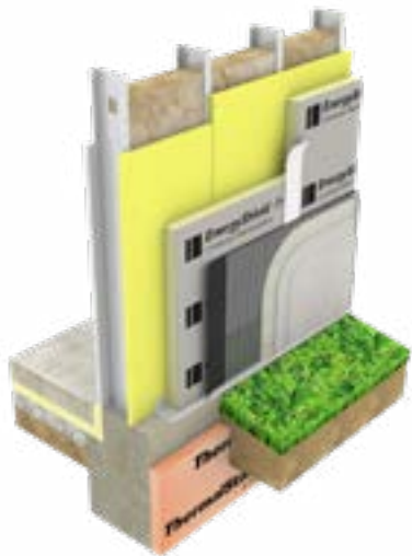
Steel studs, batt cavity insulation, glass-mat faced sheathing, EnergyShield Pro with taped joints, grade D building paper, expanded metal lath, cement plaster scratch and brown coats, stucco finish.
