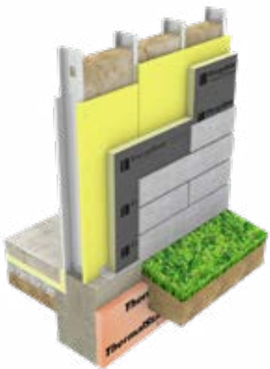
Steel studs, batt cavity insulation, glass-mat faced sheathing, EnergyShield CGF Pro with black facer side out and taped joints, metal panels installed with open joints.
