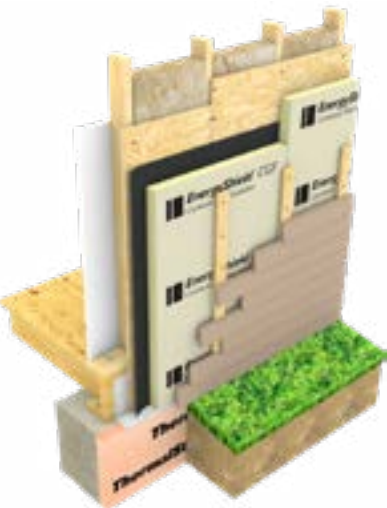
Wood studs, batt cavity insulation, wood sheathing, water resistive membrane, EnergyShield CGF, wood battens, fiber-cement siding.
