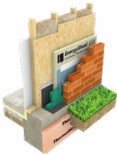
Wood studs, batt cavity insulation, wood sheathing, EnergyShield CGF, liquid applied air and moisture barrier, mortar net, brick.
