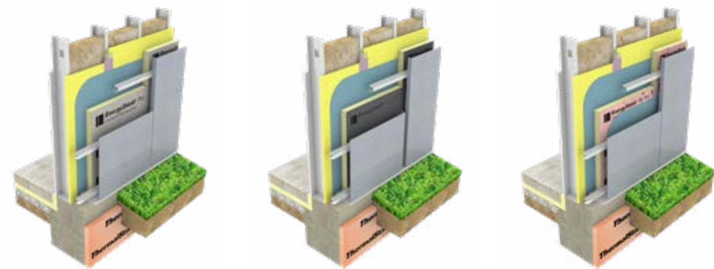
EnergyShield Pro integrates perfectly into metal panel assemblies and code compliant combinations. For open joint rainscreen applications, EnergyShield CGF Pro offers a black facer, eliminating the need for a black out fabric. Steel studs, batt cavity insulation, glass-mat faced sheathing, liquid applied air & moisture barrier, EnergyShield Ply Pro, metal panels.
