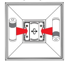
Carriage Light Solar Post Caps come with 2 Basic - AA nickel-cadmium rechargeable batteries. Premium rechargeable batteries may be desired. Batteries must be recycled or disposed of properly. Replace top by snapping it onto side panels. (Ensure the holes in the sides are matched up with the stubs on the top, fig:1) Your solar post cap is now ready to be installed onto your post.
