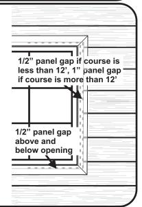
IMPORTANT: 2" Face J-trim is designed for use around openings. It can also be used in areas such as gables where the siding panels can be fastened outside of the channel. It is not designed to be used to finish the top course of siding. To finish the top course panel under the eaves, we encourage the use of the Celect Finish Trim. See the Celect Contractor Handbook for more details.
