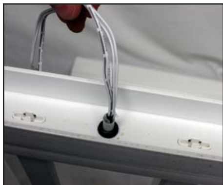
12. Rotate grommet to fully seat grommet against sub-rail
