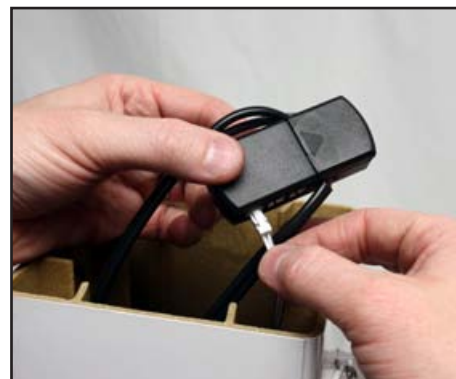
14. Insert LED Flush Pin "male" connector end into Connector Box
