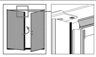
**c.** Close the inactive door panel. Ensure the weatherstrip forms a secure seal around the trim cap.
