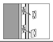
**a.** If installing new strike and deadbolt plates, remove the screws securing the old plates.
