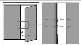
**b.** Close the active door panel and ensure the deadbolt and strike plates are aligned with the crossbore holes in the active door panel.
