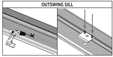
**d.** At the marked location on the sill, drill a hole **5/8" in diameter** and at least **1-3/8" deep.** Install the other plate into the sill, using two #8 x 3" screws.
