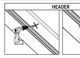
**c.** At the marked location on the header, drill a hole 3/8" in diameter and at least 1-3/8" deep. Install the header strike plate by screwing into the header, using two  $#8 \times 3$ " screws.
