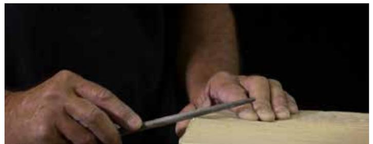
Again, fit beam end cap to beam and beam top and continue to sand as needed for final fit.
