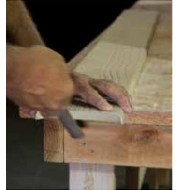
**Step 14** - To clean up corners on the bottoms of the beam, change direction of the miter to the opposite 45° angle and begin cutting around the beam bottom. Turn the beam as you go around it.
