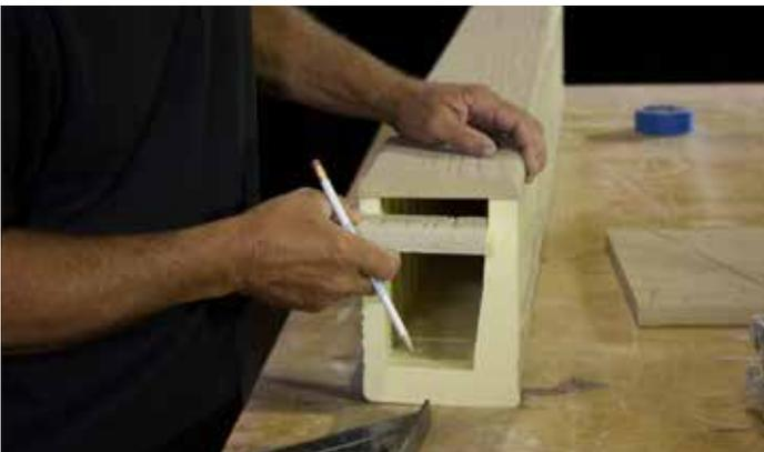
**Step 3** – Using jigsaw with fine tooth blade, cut beam and beam top to marked length (cutting all sides of the beam).
