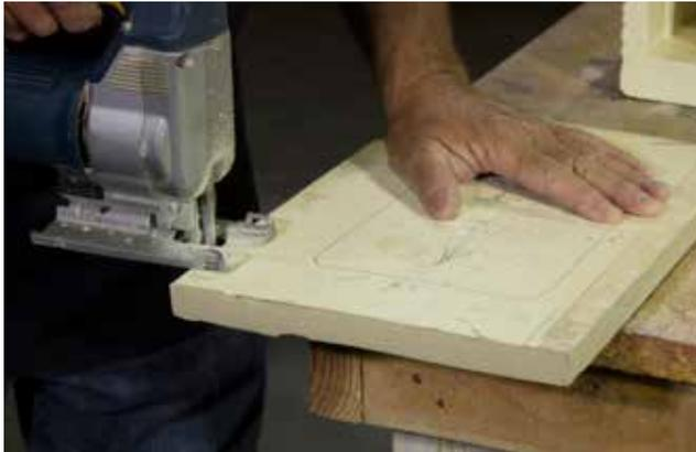
**Step 9** – After the beam end cap has been cut, move the jigsaw bevel gage to a 45° angle. You are going to miter cut the beam end cap with grain side up (make sure the miter is placed at the correct angle). Begin cutting by following the grain profile, using the painted edge as your guide
