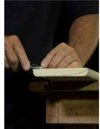
**Step 11** – Now miter the beam to accept the end cap. With the open side facing you and using the same miter angle as the beam end cap, begin cutting the beam side.
