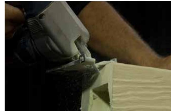
**Step 13** – Turn the beam with open side facing away from you and begin cutting the final side.
