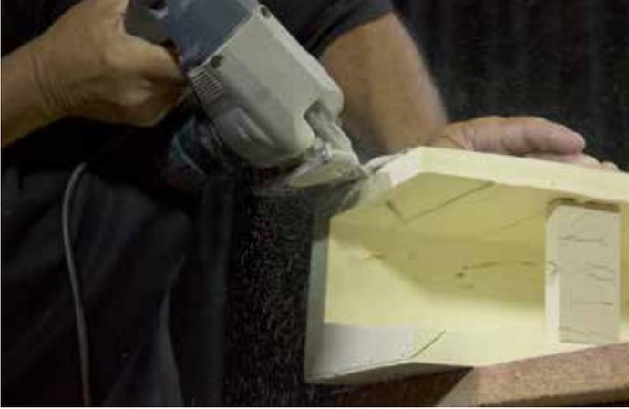
**Step 16** – Determine where the beam top and beam must be filed for beam end cap to fit securely. Using a rasp and/or file, shave the interior of the beam miter along the bottom, corners and sides of the beam. Do the same for the beam top.
