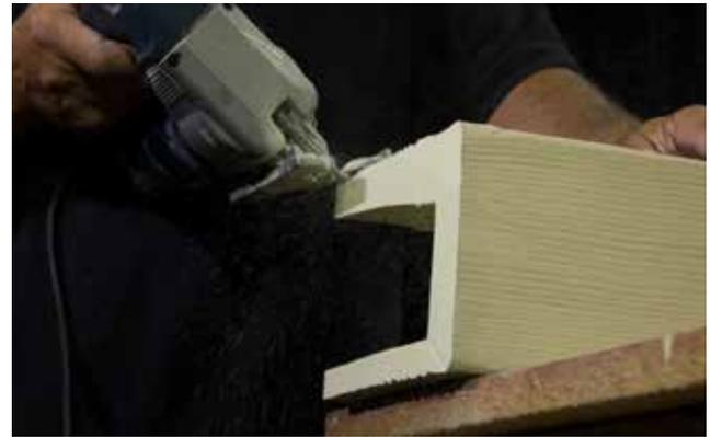
**Step 12** - Rotate the beam so the open end is sitting flat on a work surface. Start cutting the bottom of the beam at a slight angle until you can get a straight 45° angle.
