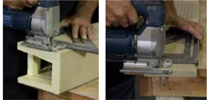
**Step 4** – Turn beam with open cavity facing upward and place the beam top on the beam to ensure the beam top and beam are at the same length.
