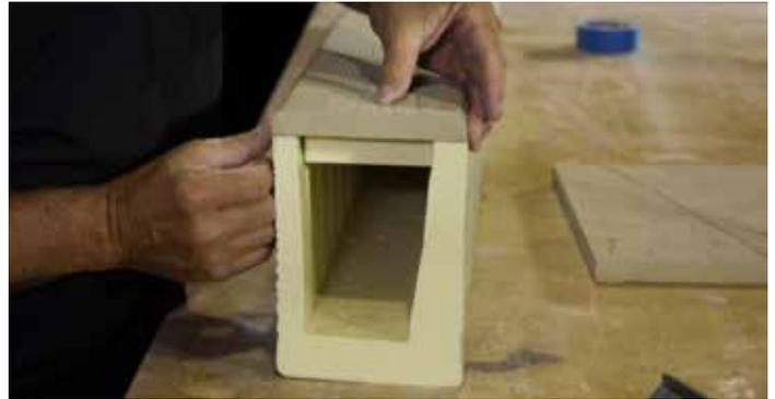
**Step 5** - After beam and beam top have been cut, tape in several places along the length of the beam or clamp beam top to the open beam.
