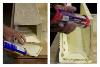
**Step 18** - Using painters tape, tape the beam end cap to the beam to secure beam end cap until adhesive dries. Once the adhesive dries (use recommended drying time specified by adhesive manufacturer), your beam is ready to paint or stain and then install.
