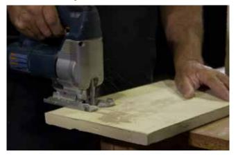
**Step 9** – After the beam end cap has been cut, move the jigsaw bevel gage to a  $45^{\circ}$  angle. You are going to miter cut the beam end cap with grain side up (make sure the miter is placed at the correct angle). Begin cutting by following the grain profile, using the painted edge as your guide.
