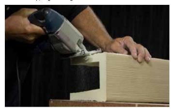
**Step 11** – Rotate the beam so the open end is sitting flat on a work surface. Start cutting at a slight angle until you can get a straight  $45^{\circ}$  angle and cut into the bottom of the beam.
