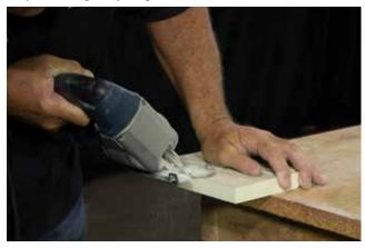
**Step 10** – Now miter the beam to accept the end cap. With the open side of the beam facing you and using the same miter angle as the beam end cap, begin cutting the beam side.
