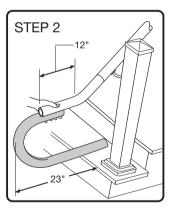
With corner now in place, determine the height of the in-line brackets on a step railing installation by holding a piece of railing in line with the elbow and parallel to the primary railing.
