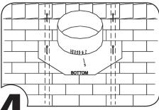
Lift tab of shingles and slide the top half of flashing under shingles and secure with nails as shown.
