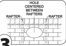
After finding the general location of turbines, (see location drawing on the back of this page), mark a hole on shingles between the rafters. Cut hole as marked. Note: Turbines may be positioned over a rafter, however this will result in a slight decrease in efficiency. Do not cut the rafter.
