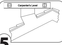
Rotate top of elbow to level position by turning counter clockwise.
