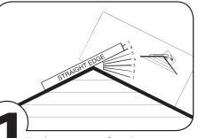
To determine roof pitch, use gauge on carton flap. Place on peak of roof and position straight edge as shown. Read roof pitch from printed gauge parallel to bottom of straight edge. This turbine is designed to fit 1/12 to 7/12 roof pitches.
