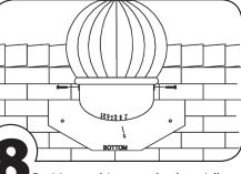
Position turbine on the base/elbow assembly. Line up the predrilled holes in sure to insert screw thru the external brace, the brackets and base and fasten with sheet elbow and internal brace. metal screws
