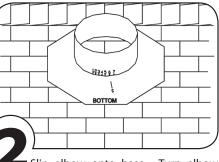
Slip elbow onto base. Turn elbow to align roof pitch number on elbow with indicator line on base and secure with three (3) sheet metal screws provided.
