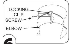
Place locking clamp across seam and tighten with included screw.
