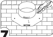
Seal the adjusting seam and the base/elbow connection seam on inside with roofing cement. Seal locking clamp holes and all exposed nails with roofing cement.
