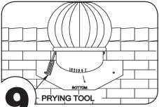
After installing check to see that the turbine turns freely. In transportation it may have shifted slightly. If necessary, minor adjustments may be made by gently prying lowest point of turbine upward to remove any wobble.
