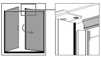
**c.** Close the inactive door panel. Ensure the weatherstrip forms a secure seal around the trim cap.
