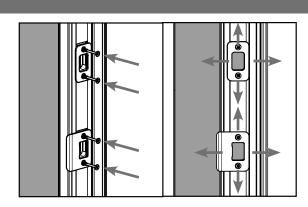
**c.** Replace the screws securing the strike and deadbolt plates with #8 x 3" screws. If the plates are misaligned, loosen the screws and adjust the location accordingly.
