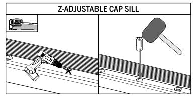
**d.** At the marked location on the sill, drill a hole **5/8" in diameter** and at least **1-3/8" deep.** Install the lower bolt receiver by tapping into the sill with a rubber mallet.
