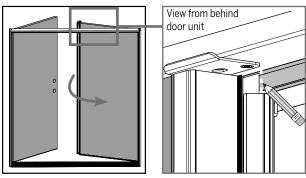
**a.** Close the inactive door. Make a mark at the location where the trim cap contacts the weatherstrip.
