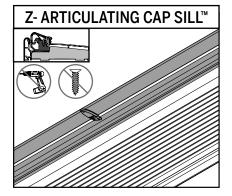
**NOTE:** If using a Z-AC sill, **no drilling is necessary** as the bolt receiver is preinstalled.
