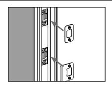
**b.** Install the new hardware into the retainers by tightening the screws through the holes in the plates.
