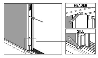
**b.** Press and engage the upper and lower bolts so the bolt pins come in contact with the header and the sill. Mark these points of contact.
