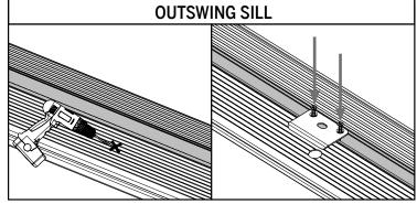
**d.** At the marked location on the sill, drill a hole **5/8" in diameter** and at least **1-3/8" deep.** Install the other hurricane plate into the sill, using two #8 x 3" screws.
