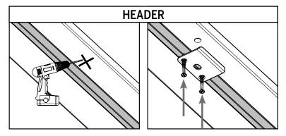
**c.** At the marked location on the header, drill a hole **3/8" in diameter** and at least **1-3/8" deep.** Install a hurricane plate into the header, using two #8 x 3" screws.
