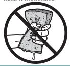
**Step 2** Wait 15 - 60 seconds before installing the corner. Adhesive should be tacky to touch. Activation time will vary depending upon room temperature, humidity and temperature of water in your pump sprayer. **Do not soak HYDROTRIM corners.**
