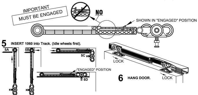
SLIDE door away from end of track (check to make sure all track screws are flat against track) and install 1060 Actuator Arm into track, with back of Actuator Arm 2-1/4" (57mm) from Jamb.
