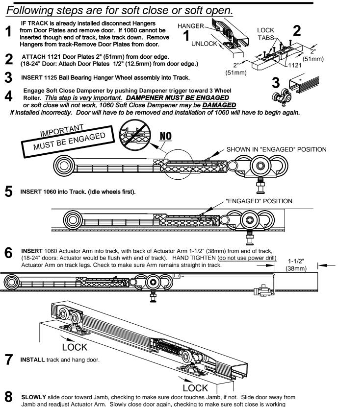
Jamb and readjust Actuator Arm. Slowly close door again, checking properly. Once confirmed, begin using door normally.
