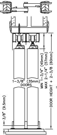
The finest bypass hardware sets you can buy. Ideal for those luxury homes or commercial installations where quality, trouble free, long life is a necessity. Precision extruded aluminum track features Johnson's line-design fascia to hide fingerprints or to hold paint if desired. Tricycle hangers ride smoothly on convex shaped rails with a single point contact and are adjustable for height. Available package sets to 8', bulk by component with track to 16'.
