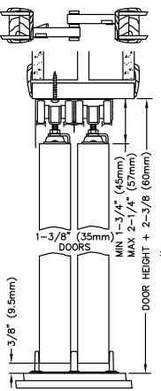
The finest bypass hardware sets you can buy. Ideal for those luxury homes or commercial installations where quality, trouble free, long life is a necessity. Precision extruded aluminum track features Johnson's line-design fascia to hide fingerprints or to hold paint if desired. Tricycle hangers ride smoothly on convex shaped rails with a single point contact and are adjustable for height. Available package sets to 8', bulk by component with track to 16'.
