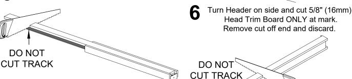
Turn Header over and cut Tracks 1-3/8" (19mm) shorter than wood Header.
