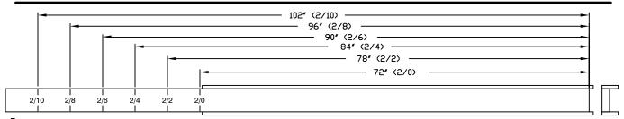
Mark Header and Side Nailers for door size.
