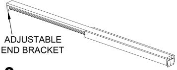
3 Cut through WOOD part of header only at mark.
