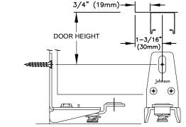
**MARK LOCATION** of Jamb Bracket (1711) on jamb. Fasten 1711 in place with one #8 X 1-1/4" (32mm) flat head screw.
