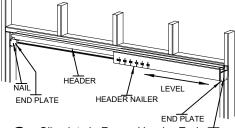
3 Slip slots in Frame Header End NAIL Plates over nails in side jambs.
