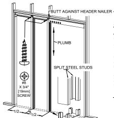
4 Slip fingers on floor Plates into the reinforcing strips of Split Steel Studs as shown. Butt Split Steel Studs against header nailer strips and screw into place.
