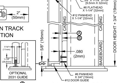
(A) GAP BETWEEN 1-3/4" (45mm) DOOR AND CASING IS 1/4" (6.4mm) (B) GAP BETWEEN 1-3/8" (35mm) DOOR AND CASING IS 7/16" (11mm)
