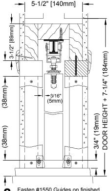
Fasten #1550 Guides on finished split jambs at door bottom so door is held in center of opening without binding.
