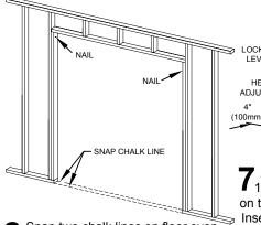
Snap two chalk lines on floor even with side jambs as shown.
