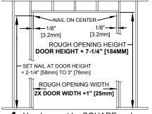
Header must be SQUARE and PLUMB with studs and LEVEL.
