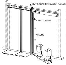
Slip fingers on floor Plates into the reinforcing strips of Split Jambs as shown. Butt split jambs against header nailer strips and screw in place.
