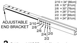
Cut through WOOD part of header only, on desired door size marking.
