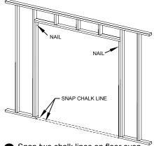
2 Snap two chalk lines on floor even with side jambs as shown.
