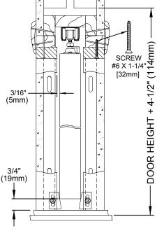
Fasten #1550 Guides on finished split jambs at door bottom so door is held in center of opening without binding.
