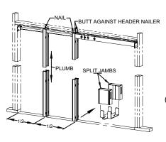
Slip fingers on floor Plates into the reinforcing strips of Split Jambs as shown. Butt split jambs against header nailer strips and nail in place.
