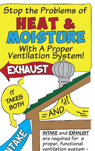
**EXHAUST VENTS** allow **HEAT** and **MOISTURE** out of your attic area. INTAKE VENTS allow fresh air into your attic area.
