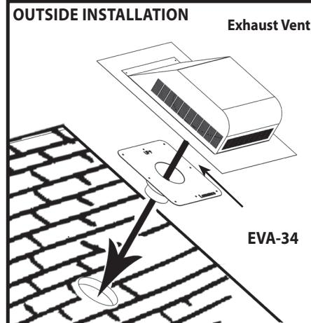
exhaust hose adapter throat. Fasten the base to roof decking with roofing nails, keeping heads of nails under shingles where possible.
