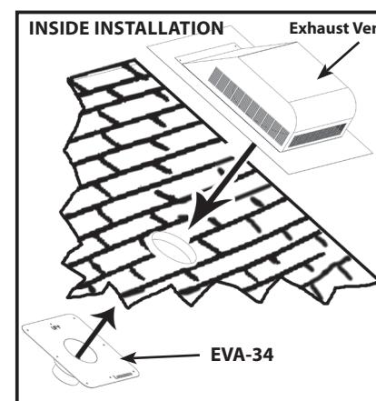
**SOFFIT MOUNTING** **Note:** We are aware that at times the exhaust hose is vented through an opening at the soffit. The EVA-34 will also work great in this application. Simply mount the flat face of the EVA-34 over the soffit opening, secure using screws in the pre-molded holes, and finally connect the exhaust hose to the adapter.
