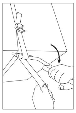
3 Keep tail horizontal to load strap and pull handle to apply tension. Advance tail through slot and repeat step 3 until buckle is closed.
