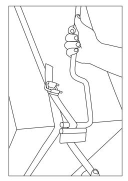
1 Feed tail of strap over bar and back through slot.
