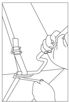
2 Brace tool against edge of load, remove slack and pull tail upward.
