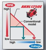
The DC Brushless Motor is more powerful, quieter and lighter than the conventional motors. Also the inverter circuit on the motor adjusts RPM to extract the maximum performance depending on the voltage level.
