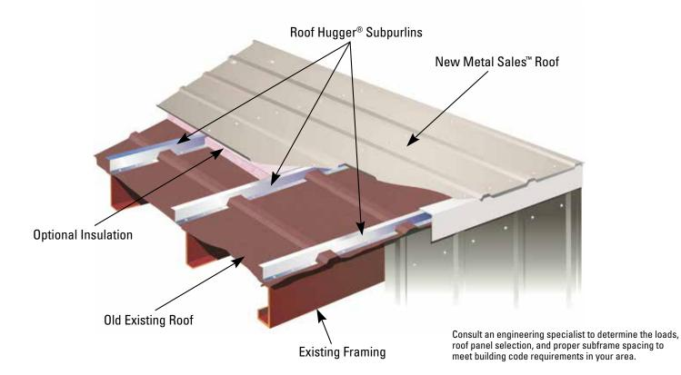
Roof Hugger components nest over the existing sloped roof panels and are compatible with the most popular Metal Sales roof profiles. Choose the re-roof solution appropriate for your retrofit needs with exposed fastened or standing seam panel options. Consult your Metal Sales representative for assistance in making your selection.
