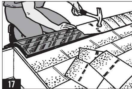
17 Nail all cap shingles in place using nails long enough to completely penetrate roof sheathing by 1/4".
