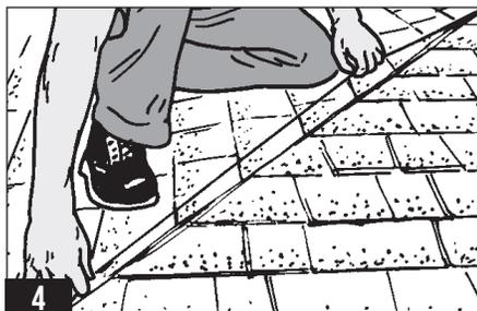
Snap two parallel chalk lines 2 1/2" apart along entire hip (1 1/4" on each side of center). Cutting away shingles on these lines with a roofing knife will make following steps easier.
