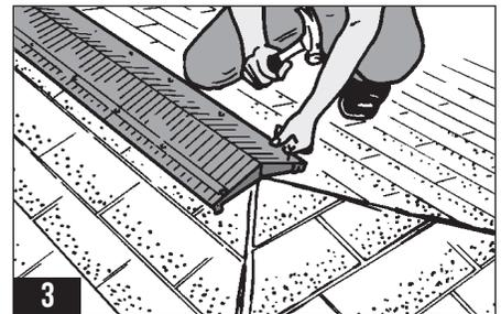
If your roof has a ridge, install RidgeMaster Plus along entire ridge from hip joint to hip joint. See RidgeMaster Plus installation, but do not install ridge cap shingles on top at this time.
