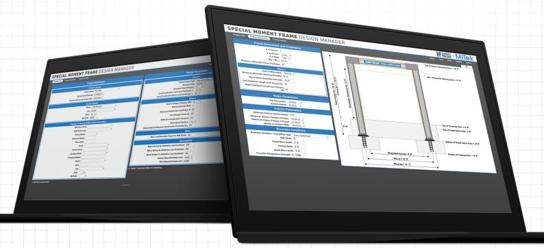
The new Hardy Frame SMF Design Manager includes three tabs – **Project Design Information,** Frame Geometry and Frame Loads.
