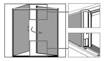
**a.** Close inactive door panel and engage both the upper and lower bolts to ensure they fit into the bolt receivers smoothly.
