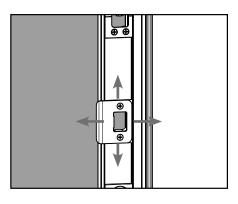
**c.** If the deadbolt actuator is not aligned, return to Step 4. If the strike plate is not aligned, loosen the screws and slightly adjust the location of the plate.
