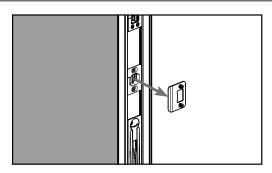
**a.** If installing new hardware, unscrew the securing screws and remove the old strike plates from the retainer.
