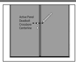
**a.** Determine the deadbolt crossbore centerline of the active door panel and mark this location on the inactive door.
