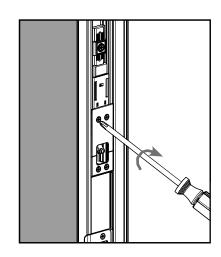
**d.** Tighten the four screws on the deadbolt actuator. **Do not overtighten.**
