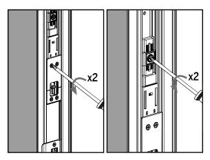
**b.** Loosen the four screws on the deadbolt actuator and actuator adjuster screw two turns each.
