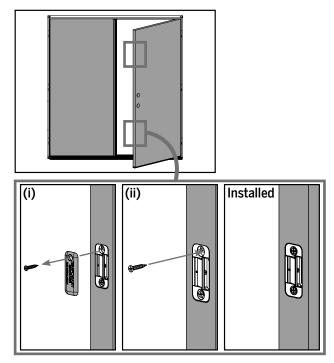
**f.** When painting and installation are complete, (i) remove the screw from the spacer on each keeper and remove the spacer. (ii) Reinstall the screw to secure it in place.
