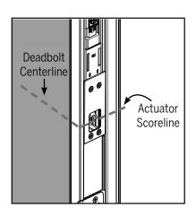
**c.** Adjust the location of the deadbolt actuator so the actuator scoreline aligns with the deadbolt crossbore centerline.
