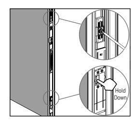
**e.** Hold down the lock pawl on the lower bolt and tighten the actuator adjuster screw to set the location of the deadbolt actuator.
