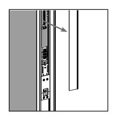
**a.** Remove the trim strip located right above the deadbolt actuator.
