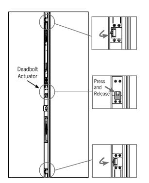
**d.** Press and release the deadbolt actuator and ensure that when the deadbolt actuator is depressed, the lock pawls move between engaged and disengaged positions smoothly.
