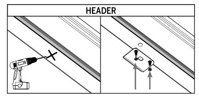
**c.** At the marked location on the header, drill a hole 3/8" in diameter and at least 1-3/8" deep. Install the header strike plate into the header, using two  $#8 \times 3$ " screws.
