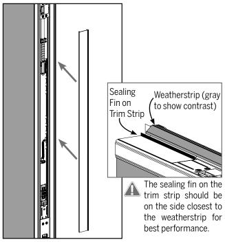
**e.** If the trim strip was removed, reinstall the trim strip so it is flush between the upper lock pawl housing and the deadbolt actuator. If necessary, cut off any excess trim strip.
