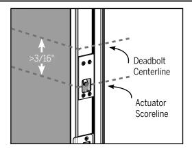
**b.** Check the alignment of the deadbolt actuator with the deadbolt crossbore centerline. If it is misaligned by more than 3/16", adjust the location of the deadbolt actuator as detailed in Step 5. If they are aligned, skip to Step 6.
