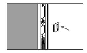
**b.** Install the new hardware into the retainers by tightening the screws through the holes in the new strike plate.
