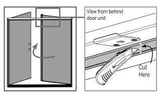
**b.** Open the inactive door. Using a utility knife, make a slit in the weatherstrip along the mark made.
