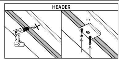
**c.** At the marked location on the header, drill a hole **3/8" in diameter** and at least **1-3/8" deep.** Install the header strike plate by screwing into the header, using two #8 x 3" screws.
