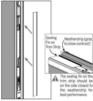
**e.** If the trim strip was removed, reinstall the trim strip so it is flush between the upper lock pawl housing and the deadbolt actuator. If necessary, cut off any excess trim strip.
