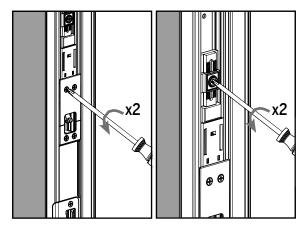
**b.** Loosen the four screws on the deadbolt actuator and actuator adjuster screw two turns each.
