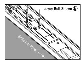
**b.** Remove the orange securing pins from the lower bolt and replace them with #8 x 1-1/2" screws.
