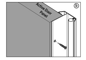
**b.** Install the screws through the predrilled holes to secure the flange snug against the face of the active door.
