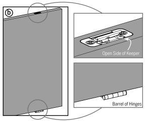
**b.** Install the spacer into each pocket as shown. The open side of the keeper must face the same side as the barrel of the hinges on the opposite door panel.
