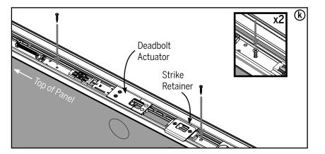
**k.** Install two #8 x 1" screws into the holes in the astragal body on either side of the strike retainer and deadbolt actuator.
