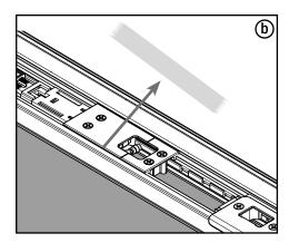
**b.** After securing the actuator, remove the tape which holds the actuator in place during installation.
