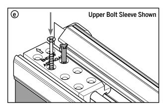
**e.** Install a #8 x 1-1/2" screw next to the popped orange securing pin on the upper bolt sleeve.
