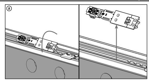
**a.** Rotate the actuator out of the astragal body toward the narrow edge of the astragal.
