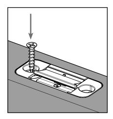
c. Secure the keeper assembly installing one of the #8 x 1" screws into each keeper.
