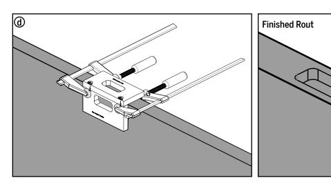
**d.** Rout the pocket using a 1/2" router bit with 5/8" diameter collar, rout slot in the door panel 7/16" deep.
