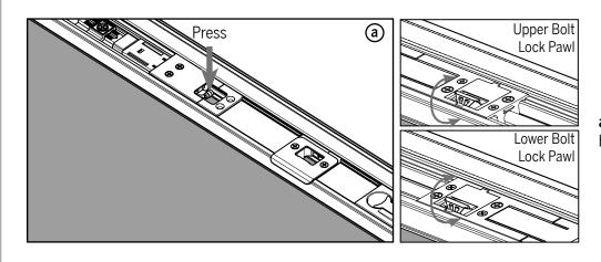
**a.** Operate the deadbolt actuator by pressing down on it. Ensure the top and bottom lock pawls move between engaged and disengaged positions.
