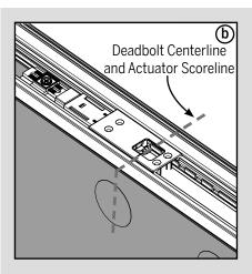
**b.** If the actuator scoreline is in line with the panel deadbolt crossbore centerline, skip to Step 9.
