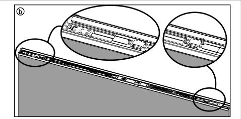
b. Press the astragal down along the length of the panel. A total of five orange securing pins will pop up around the lower and upper lock pawls, and the upper bolt sleeve.
