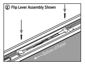
**g.** Secure the flip lever assembly with two #8 x 1-1/2" screws.
