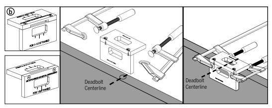
**b.** Position the deadbolt centerline to be lined up with the lower small mark on the template. Make sure to use the side of the template that matches the door panel thickness.
