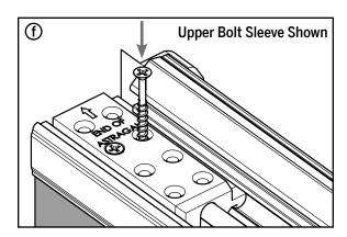
**f.** Remove the orange securing pin from the upper bolt sleeve and replace it with a #8 x 1-1/2" screw.
