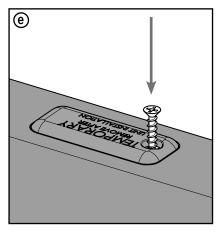
**e.** Install the second #8 x 1" screw through the spacer and the keeper into the door panel.
