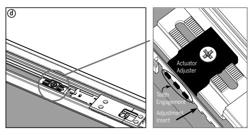
d. Ensure the teeth on the actuator adjuster engage into the rack teeth on the adjustment insert.
