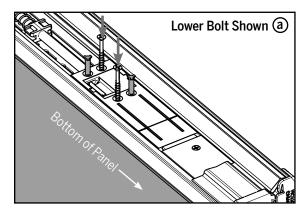
**a.** Keeping the orange securing pins in place, install  $\#8 \times 1-1/2$ " screws in the holes adjacent to the pins.
