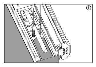
i. Install #8 x 1" screws into the holes directly above the U-notch on the astragal body.
