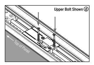
**d.** Remove the orange securing pins from the upper bolt and replace them with #8 x 1-1/2" screws.
