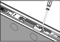
Secure the strike plate into the proper location by aligning it with the lever crossbore hole and tighten the screws into the retainer.
