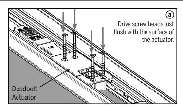
a. Drill Ø1/8" x 1-1/2" deep pilot holes at each deadbolt actuator hole. Install four #8 x 3" painted screws into each actuator hole.
