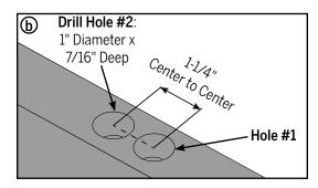
**b.** Drill a second hole 1-1/4" above the first hole. This hole will also be 1" in diameter and 7/16" deep.
