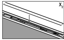
**Upper Trim Strips:** Align  $X_1$  with the top of the upper bolt and top of the upper lock pawl housing. Press down to secure. Align  $X_2$  with the bottom of the upper lock pawl housing and the top of the deadbolt actuator. Press down to secure.
