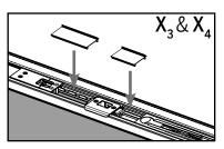
**Middle Trim Strips:** Align  $\mathbf{X_3}$  with the bottom of the deadbolt actuator and the top of the strike retainer. Press down to secure. Align  $\mathbf{X_4}$  with the bottom of the strike retainer and the top of the flip lever assembly. Press down to secure.
