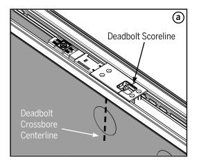
a. Check where the deadbolt actuator scoreline is positioned relative to the deadbolt centerline.
