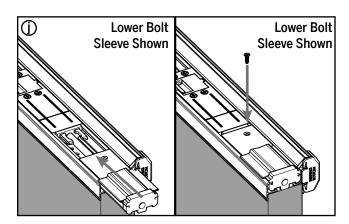
**j.** Return the bolt sleeve onto the lower bolt and reinstall the screw securing the bolt sleeve.
