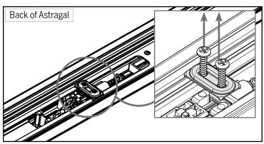
On the back of the astragal, a shipping clip secures the deadbolt actuator. Using a Phillips Screwdriver, remove the screws and discard the shipping clip.
