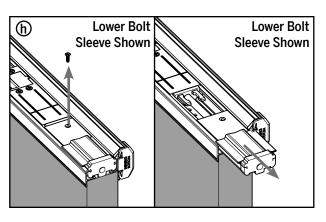
**h.** Remove the lower bolt sleeve retainer screw and slide out the lower bolt sleeve.
