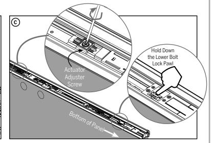
**b.** Move the actuator up or down to line up the **c.** While holding down the lock pawl on the bottom bolt, tighten
