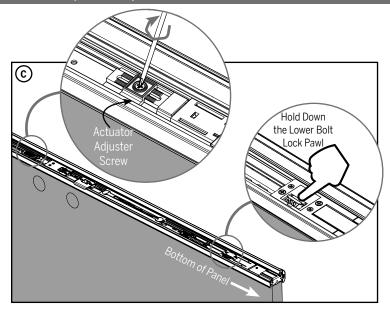
c. While holding down the lock pawl on the bottom bolt, tighten the deadbolt actuator adjuster screw.
