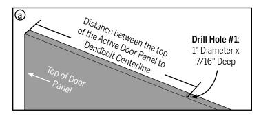
**a.** Mark the center of the rout location at the centerline of the deadbolt crossbore. Once marked, drill a hole that is 1" in diameter and 7/16" deep.
