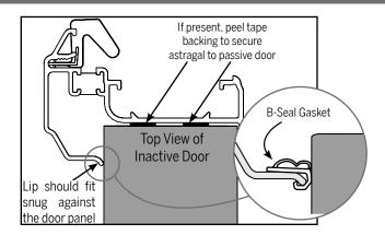
Confirm the thickness of your door panel. For door panels with thicknesses of 1-11/16", apply the available B-seal gasket to accommodate the gap between the panel face and astragal.
