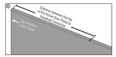
**a.** Mark the center of the rout location at the centerline of the deadbolt crossbore.
