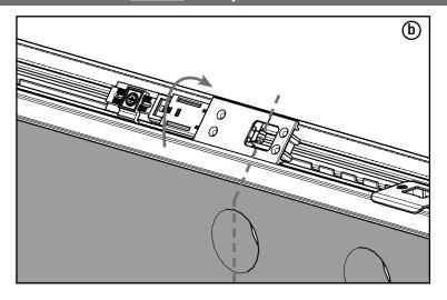
**b.** Line up the scoreline on the actuator body with the center of the inactive panel deadbolt crossbore and rotate the actuator into the astragal body, starting at narrow edge of astragal.
