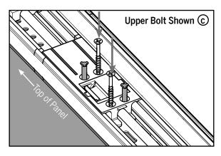
**c.** Keeping the orange securing pins in place, install #8 x 1-1/2" screws into the open holes around the upper lock pawl, next to the pins.
