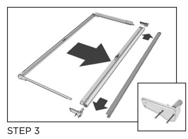
Release the tracks and remove the screen housing end caps (2 long outside screws only). Keep parts and new screen in same position after removal to ensure proper placement. Screen may make noise when tension is released.
