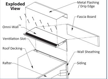
Install all Exhaust Ventilation at the SAME HEIGHT within a common attic area.
