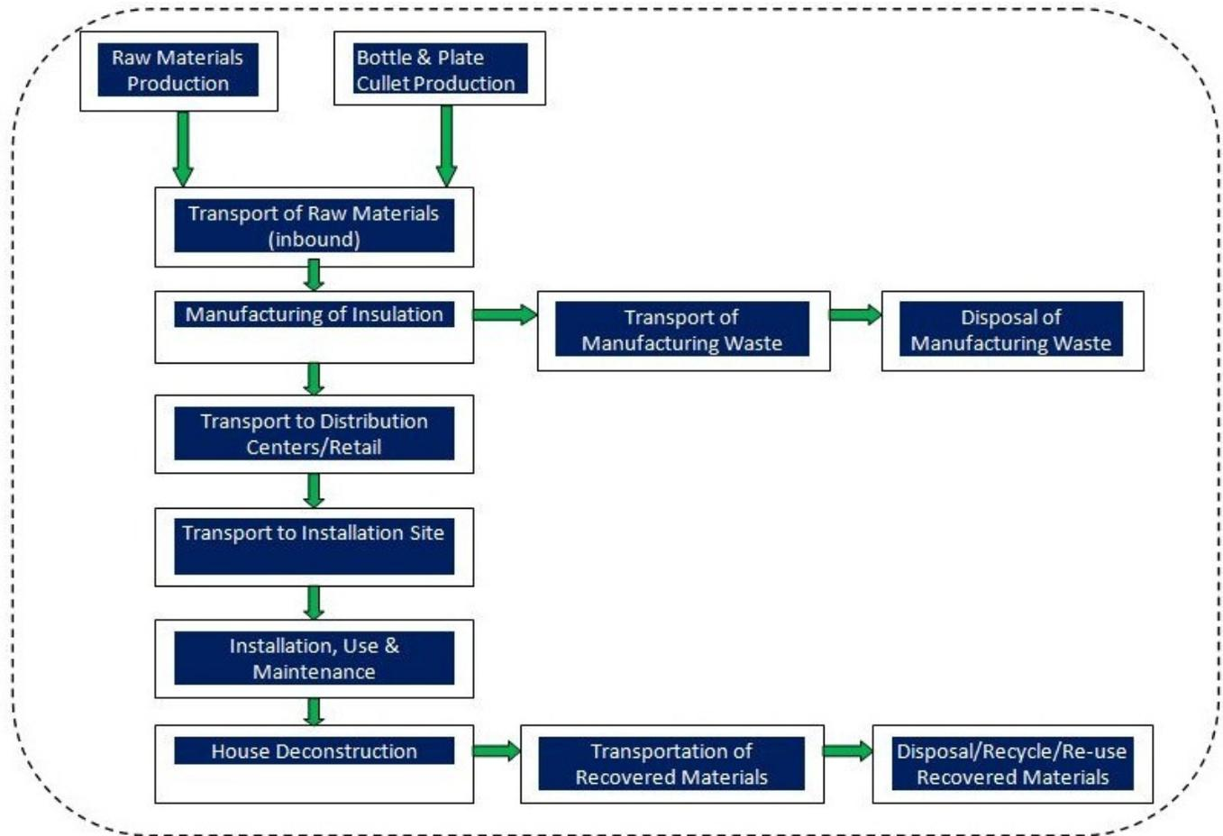
Figure 5: Process Flow Diagram for EcoTouch® Foil Faced Insulation Manufacturing
