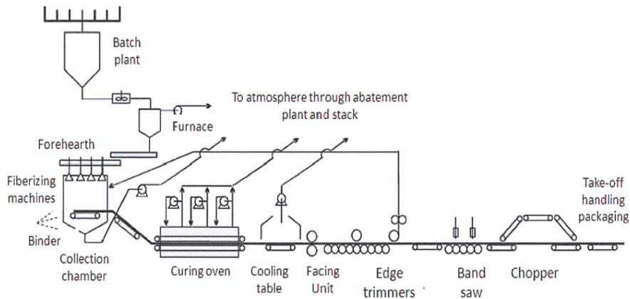
Figure 1: Manufacturing Process of EcoTouch® Foil Faced Insulation
