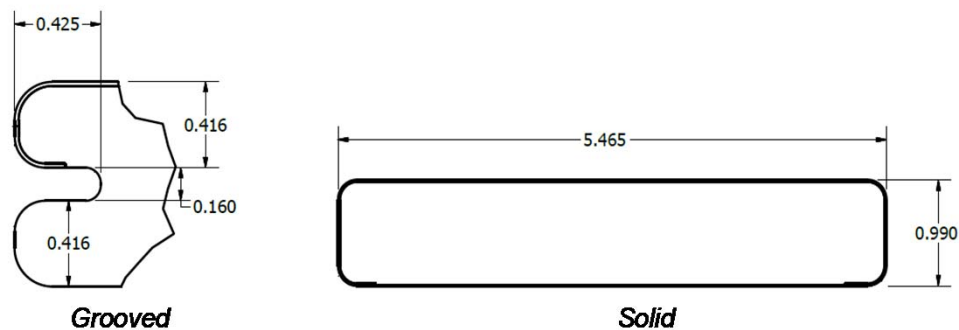
Figure 14 - Fiberon Paramount® PVC Cross-Section
