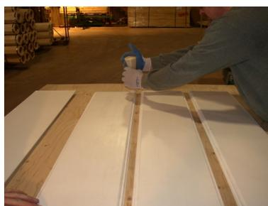
5) Lay 3 panels flat and apply adhesive to center joints.
