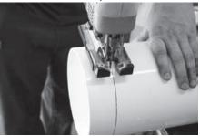
Remove the unwanted amount using a saber saw with a fine tooth blade.
