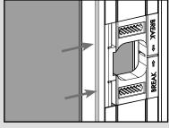
${\bf a.}$  Remove the retainers from the astragal body by pushing the tabs in and rotating the retainer out.
