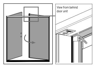
**a.** Close the inactive door. Make a mark at the location where the trim cap contacts the weatherstrip.
