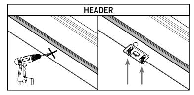
**c.** At the marked location on the header, drill a hole **3/8" in diameter** and at least **1-3/8" deep.** Install the header strike plate into the header, using two #6 x 1-1/2" screws.
