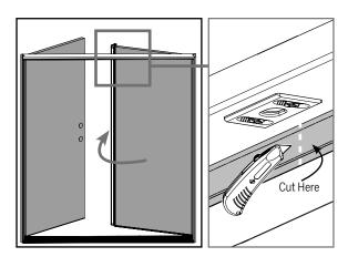
**b.** Open the inactive door. Using a utility knife, make a slit in the weatherstrip along the mark made.
