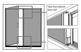
**a.** With the inactive door closed, engage both the upper and lower bolts to ensure they fit into the bolt receivers smoothly.
