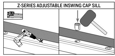
**d.** At the marked location on the sill, drill a hole **5/8" in diameter** and at least **1-3/8" deep.** Install the lower bolt receiver by tapping into the sill with a rubber mallet.
