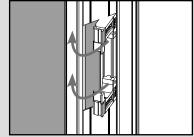
**c.** Break retainer in half using the bend lines. Return the two pieces of the retainer to the astragal and adjust to fit the larger hardware.
