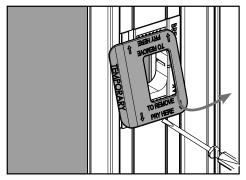
**a.** When you are ready to install the hardware on the door, pry off the dummy strike plates using a flathead screwdriver.
