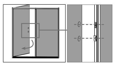
**b.** Close the active door panel and ensure the deadbolt and strike plates are aligned with the crossbores on the active door panel.
