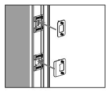
**b.** Install the strike and deadbolt plates by screwing into the retainers.
