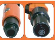
**TOOL/POLE CONNECTION** The new poles have an internal rod, when activated by pushing on the pole sleeve triggers the new Viper.
