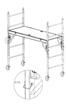
7) Insert the caster into the outrigger and attach the outrigger to the frame leg using two 2" snap pins. The caster on the outrigger should be level with the casters on the ladder frame.
