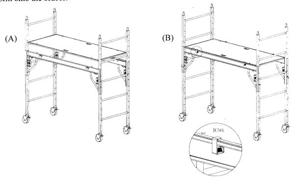
5) The platform height can now be easily adjusted. By standing at the end of the unit, disengage a lock pin with each hand. The arm braces and platform can now be moved up or down on the frame. When at the preferred height, release the lock pins and move the platform up or down until the lock pins snap into the nearest hole. Adjust the opposite end in the same way.
