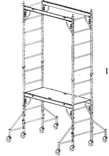
10) Attach the second level arm braces one at a time as described in step 2 and position them to the top of the second level ladder frames.
