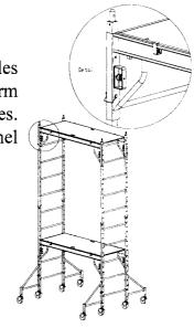
12) Set the guard rail end panel on the second level ladder frame and secure with 2" snap pins. Repeat for the opposite end of the scaffold unit.
