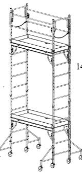
14) Install the four toe board clips onto the ladder frames and then place the toe board into the clips. Repeat step for the second platform.
