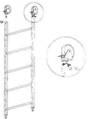
2) (A)Turn the frames right side up and engage the lock on the casters. While holding one end frame with one hand use your other hand to pull back the lock pin on the arm brace and engage the "U" channel over the frame leg. (B)Then release the lock pin and slide the arm brace up or down on the frame leg until the pin snaps into a hole. Repeat for the opposite end of the brace and second end frame.
