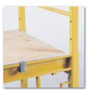
Edge banding protects all four sides without using rivets, screws or staples. Handle holes on each side make for ease in handling. Platform is held in place with four spring-loaded retaining clips.
