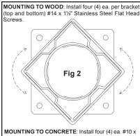
MOUNTING TO CONCRETE: Install four (4) ea. #10 x 13/4" Tapcon Screws into bottom bracket. Use four (4) wood mount screws (above) for top mounting plate.
