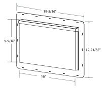
Face of mount is uncut for on-site fabrication.
