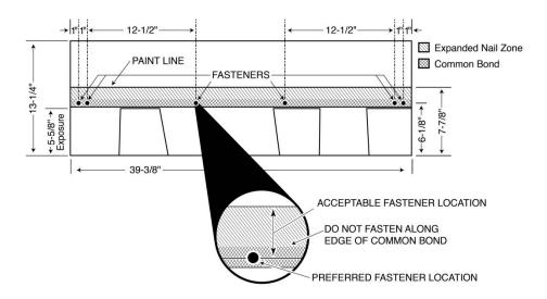
This document is not intended nor should it be construed to modify or alter the terms of the TAMKO Fiberglass/Asphalt Shingle Limited Warranty and Arbitration Agreement. **Use of this fastening pattern DOES NOT qualify for TAMKO's High Wind Application Limited Warranty.** To qualify for the High Wind Application Limited Warranty, place fasteners in the common bond area and spaced as shown in the illustration above.
